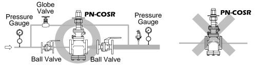
11. External secondary pressure-sensing line (when required)
