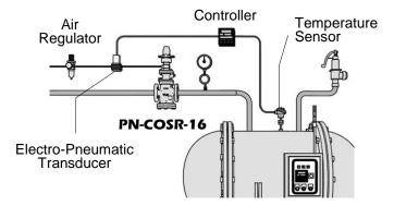
Automatic control is possible when the **PN-COSR-16** is used with a controller. However, an electro-pneumatic transducer is required in order to control the air for operation. The wiring, etc. should be carried out according to the instruction manual for the controller, the electro-pneumatic transducer, or related devices.
