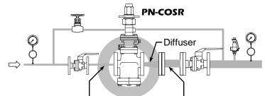
Straight-run piping lengths (d = pipe diameter): Upstream = 10 d or more; Downstream = 15 d ore more
