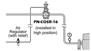
When operating the **PN-COSR-16** remotely by manual operation, an air regulator (with relief function) that adjusts motive air pressure is required. Adjust the set pressure with the air regulator while checking the pressure gauge on the secondary side.
