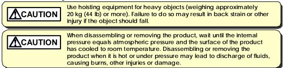
It is a recommended practice to dismantle and inspect the **PN-COSR-16** once a year for preventive maintenance purposes. It is especially important to perform an inspection immediately after the initial run of a new line or before or after equipment such as a heater is out of service for a long period of time. (Installation, inspection, maintenance, repairs, disassembly, adjustment and valve opening/closing should be carried out only by trained maintenance personnel.)
